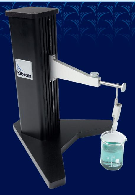
The base support has M6 mounting holes for securing on the Microtrough Gx base, or any standard optical breadboard. When used with older MicrotroughX series the dipper is on a separate stand.
