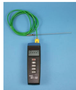
MIN/MAX digital thermometer with add. temperature sensor
